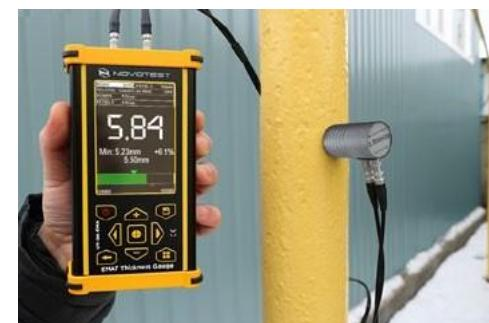
EMA technology generates waves directly in the material (ferromagnetic and paramagnetic), thus allowing measurements to be carried out under the coating, with a poorly prepared surface or even air gap, which may not be feasible with traditional methods.
