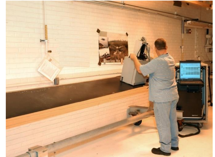
Flash Thermography Inspection of V-22 Proprotor at FRC-E
