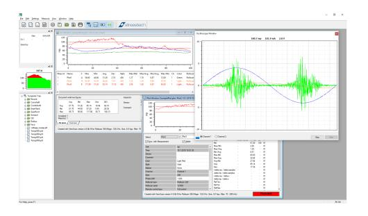
Rollscan 350 can be completed with MicroScan software for material analysis. The system provides analysis of data with freely adjustable analyzing frequency filter (RMS, peak value, peak position, FWHM, amplitude spectrum, integral of the bursts, pulse height distribution). Using MicroScan you can:
