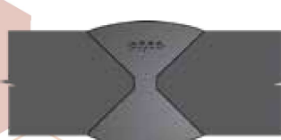
30 Porosity in Double Vee (sub-surface) UT, RT
