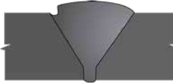
59 Incomplete Groove Weld (crown area) VT, MT/PT, UT, RT
