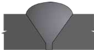
74 Excess Crown in Single Vee VT
