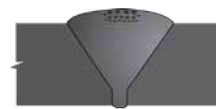
32 Porosity in Single Vee (surface breaking) VT, MT/PT
