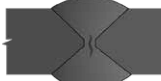
15 Centerline Crack in Single Vee (sub-surface) UT, RT
