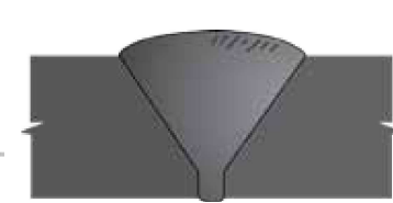
92 Chipping Hammer Marks on Single Vee, VT, RT
