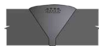
30 Porosity in Single Vee (sub-surface) UT, RT
