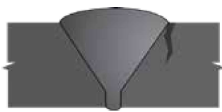
10 Toe Crack in Single Vee MT/PT, UT
