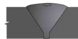
20 Crater Crack (crown stop-start area) MT/PT, UT
