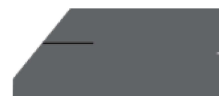
51 Lamination in Weld Prep MT/PT, UT
