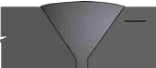
50 Lamination in Single Vee (base metal) UT
