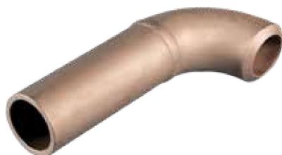
L/R 90° ELBOW TO PIPE 2" SCH160 (.344" T) #P104
