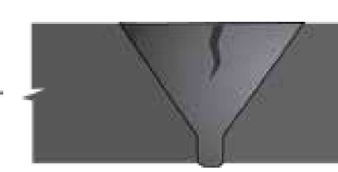
16 Circumferential Crack in Single Vee, flush crown MT/PT, UT
