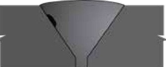
52 Lack of Fusion in Single Vee (crown area) UT
