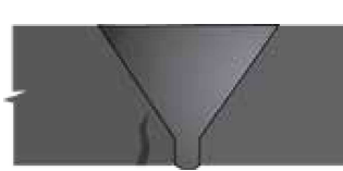
19 Base Metal Crack in Single Vee (bottom HAZ area) MT/PT, UT
