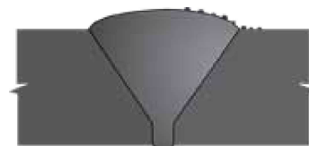
90 Weld Splatter on Single Vee, VT, RT
