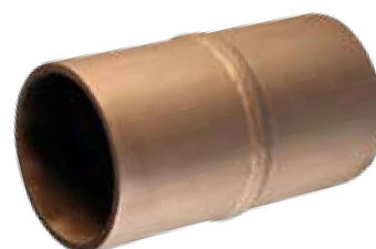
WELDED PIPING 4" SCH160 (0.53" T) x 8" #P109
