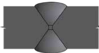
57 Incomplete Root Penetration in Double Vee, VT, RT
