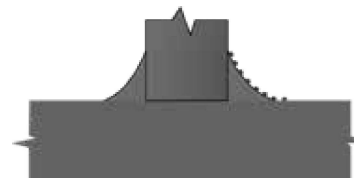
91 Weld Splatter on Filler VT, RT
