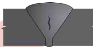
15 Centerline Crack, Single Vee (sub-surface) UT, RT
