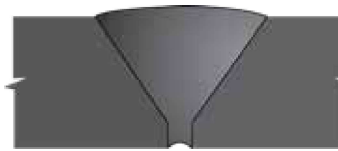
70 Root Concavity in Single Vee VT, RT
