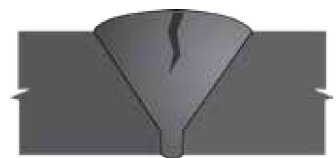
14 Centerline Crack, Single Vee (surface breaking) MT/PT, UT, RT
