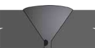
36 Slag Inclusion in Single Vee (root area) UT, RT
