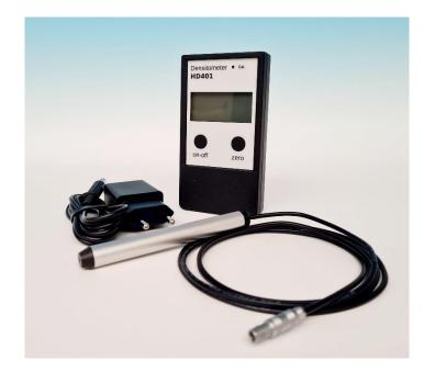
The WILNOS handheld densitometer HD401, article no. 23 13 02, is specially developed for measuring the density of technical X-ray films. It is focused on measuring accuracy, linearity as well as ease of use. The device can be used in battery and mains operation and is therefore equally suitable for stationary and mobile use. It has a large backlit display. In mobile use, it scores with its low weight and convenient device dimensions.
