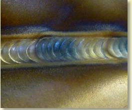
The ferrite level is important to assure minimum exposure to solidification cracking when depositing austenitic stainless
