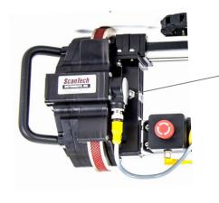
Simple set screw to make the drive section rigid or non rigid for pipes or tanks.
