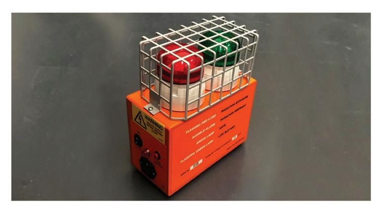
The 500B GAMMA-ALARM is a portable, battery powered alarm system designed for Gamma-ray inspection areas utilizing an internal GM tube. The alarm will indicate audibly before and visually when an exposure is in progress. The pre-set threshold level is typically 7.5µSv/h unless otherwise specified. The 500B GAMMA-ALARM can also be used anywhere in the world as it can accommodate a supply voltage from 100V AC to 240V AC 50/60Hz.
