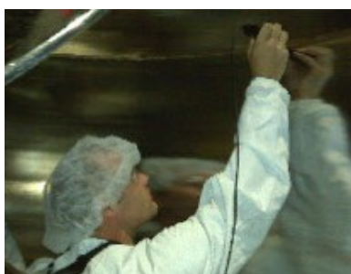
Stainless Steel Pharmaceutical tank inspection using standard Lizard® probe arrays
