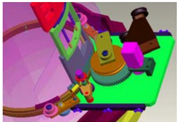
CAD image of the robotic manipulator used for the automated scanning of the Lizard Versatile Array sensor. The Lizard's ability to utilise two dimensional array configurations were essential to the application due to the access limitations on site
