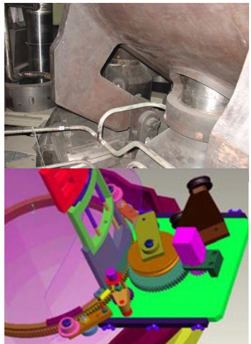
Nuclear PWR application and CAD presentation of robotically deployed Lizard® array
