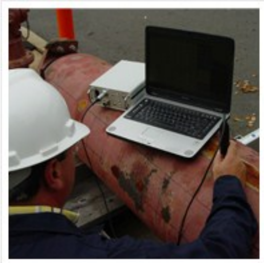
Standard Inspection using the Lizard® M8 and LP600 Lizard Probe
