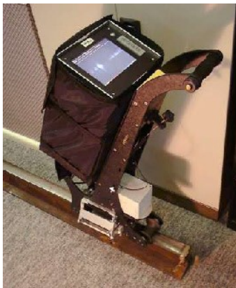
Lizard® FGI Pedestrian Unit for the Inspection of Rail
