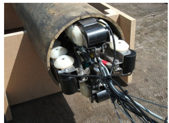
The Lizard® FGI pipe inspection system deployed in a 10 inch pipe for the single pass identification of defects on the inside and outside pipe wall
