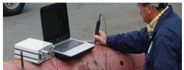
The Lizard M8 in use performing an inspection through a protective coating
