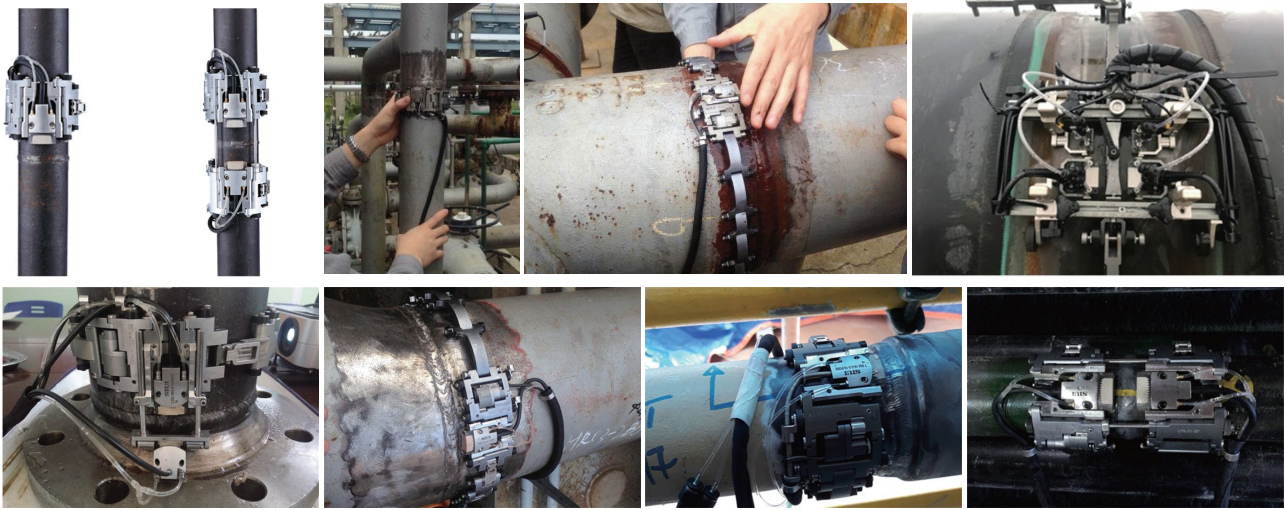
Phased array butt weld inspection crawler
