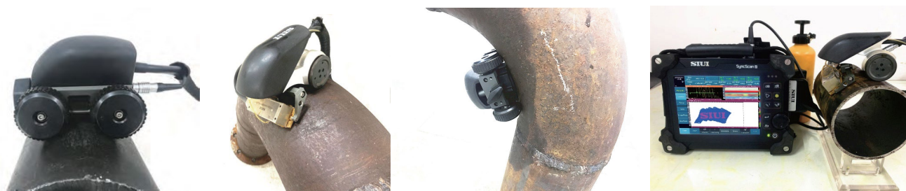
Corrosion mapping crawler
