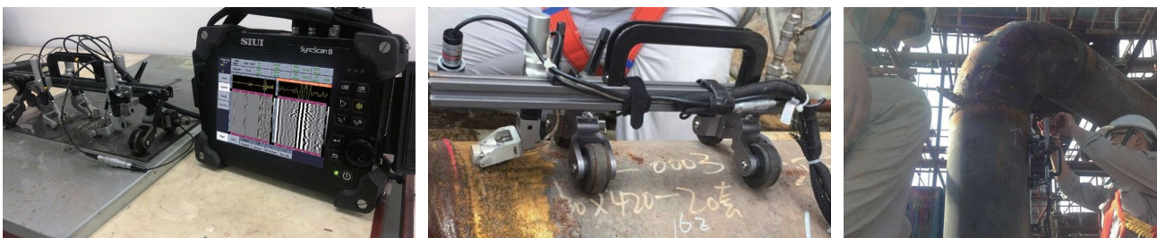
Phased array & TOFD crawler
