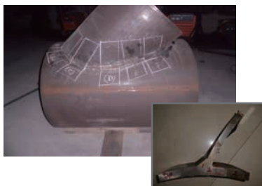
Y-shape weld joints cut from a huge pipe
