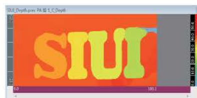
C Scan In-Depth, showing echo depth, can be used for simple corrosion inspection.
