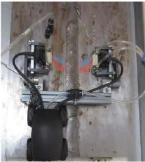
Dual-side Butt Weld Inspection
