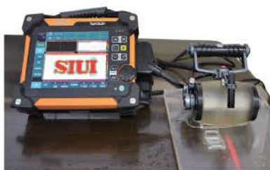
Linear Scan Image on Flat Panel Engraved with SIUI logo.
