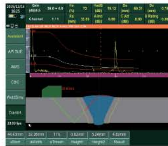
Crack Height Measurement
