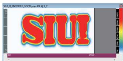
C Scan In-Amplitude, showing echo amplitude
