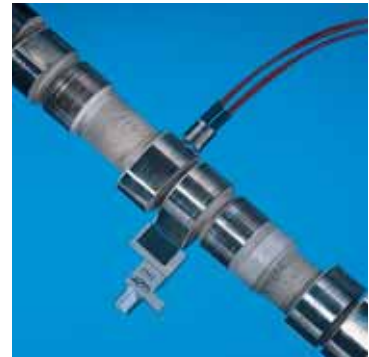
Overheating when grinding and cracks on camshafts
