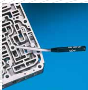
Crack detection on complex structures
